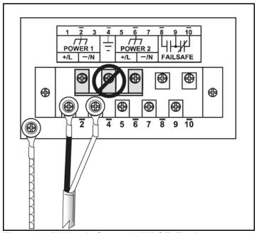
Figure 22: Dielectric Strength (HIPOT) Testing
